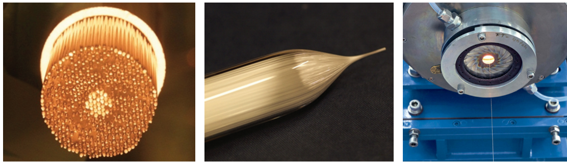
(a) The preform, a hand-assembled capillary stack (for kagome fibre). [283] (b) The cane, a millimetre-sized intermediary to be re-drawn. [283] (c) HC-PCF leaving the furnace, ready to be coated. [284]
